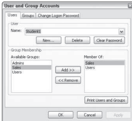
Figure 22-16: Assigning users to groups makes controlling object permissions much easier for the system administrator.
