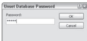
Figure 22-4: You can remove a database password by entering the password in the Unset Database Password dialog box.
