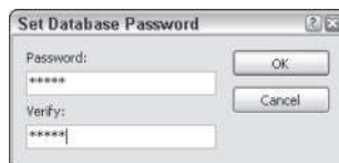
Figure 22-3: Creating a database password is the simplest way to secure your database.
