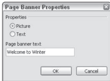
Figure 23-17 A page banner being defined. A page banners will display as a picture only if a theme is assigned to a page.
